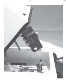
Figure 11: 2025i – Inserting an External Temperature Probe into the Sampling Chamber
