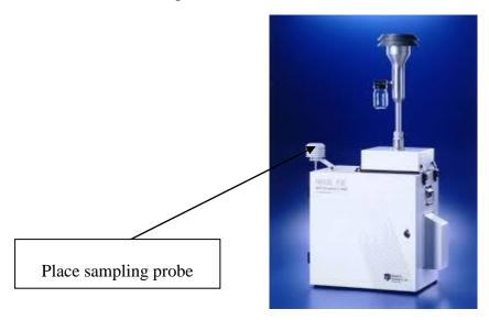
**Figure 8: Ambient Temperature Sensor**
