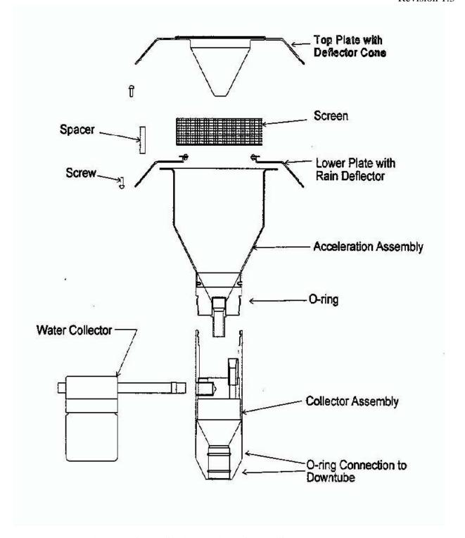
Figure 1. Cross-Sectional View of PM<sub>10</sub> Sampler Inlet Head
