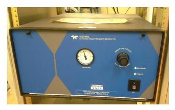
Fig. 1: Front panel of the T701H Zero Air Generator.
