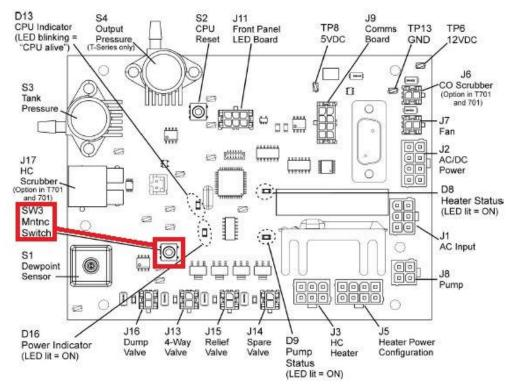
Fig. 3: T701H Control Board, maintenance mode button location
