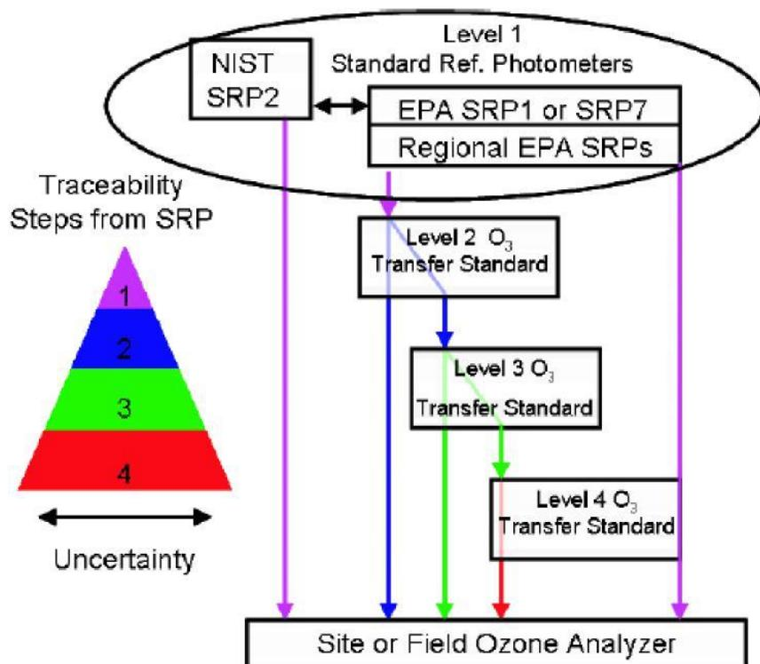
**Figure 1. Transfer Standards for Calibration of Air Monitoring Analyzers for Ozone**
