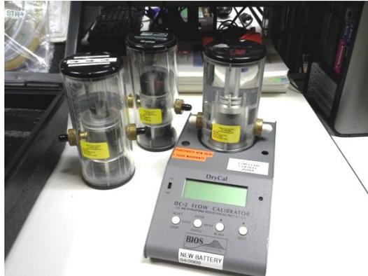
**Figure 3: BIOS DryCal flow measuring device.**
